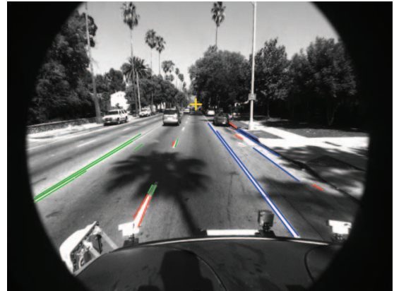
Figure 4. Selected and eliminated line segments according to their locations. Vanishing point is indicated with a yellow cross sign.
